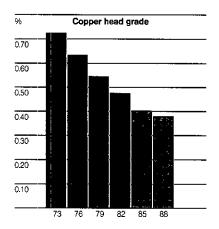
some extent this decline in grades is counterbalanced by a decrease in the waste to ore ratio as external waste material is removed to access the orebody.
